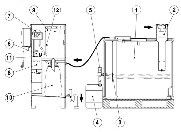
The oil-containing condensate can be supplied under pressure to the BEKOSPLIT® 12. The overpressure is relieved in the pressure relief chamber (2), without causing turbulences in the preseparation container (1).
