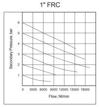
Flow graphs are for 40µm filterations only
