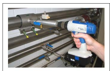
Drilling with drilling jig Order no. 0530 1108
