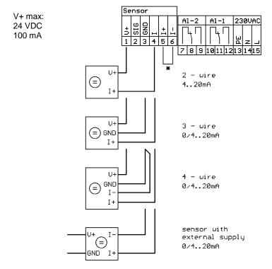
\* A bridge circuit is inserted ex factory . For signal transfer please remove the bridge circuit and attach the connection cables. Attention: Current loop has to be closed!
