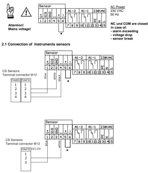
\* A bridge circuit is inserted ex factory . For signal transfer please remove the bridge circuit and attach the connection cables. Attention: Current loop has to be closed!
