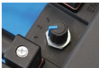
Unique switch allowing user to set -20°C, -40°C and -74°C DMC operation.
