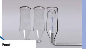
Prior to filling, bottles are cleaned and blown out with compressed air for drying. Oil in the compressed air would accrete on the walls of the bottle and subsequently enter the product once filled. Oil free compressed air is an essential production factor for safe, quality product.
