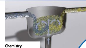
For the mixing of different materials, compressed air is employed. Materials to be mixed are blended in a silo by means of compressed air. The prerequiste condition for a perfect end product is processed and oil free compressed air
