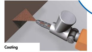
During painting / coating applications, compressed air is, amongst other uses, employed to transfer the paint from the spray gun to the carrier material. Oil contaminated compressed air leads to a variety of surface defects.
