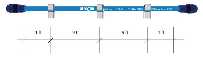
For all pipe sizes ]h]g f YWca a YbXYX hc ]bg/U` three brackets per 20ft length positioned as shown above"
