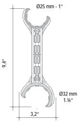
PURESTREAM wrench allows a correct nut tightening without any damage of the fitting. The wrench is exclusively designed for PURESTREAM by Aircom system.
