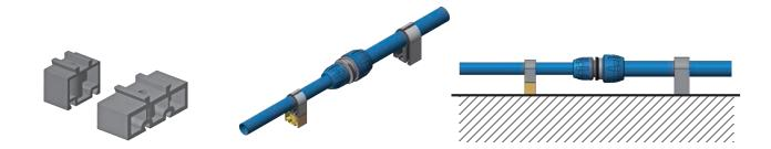
Brackets are positioned avoiding any contact with fittings or other accessories liable to block the sliding of the pipe.
