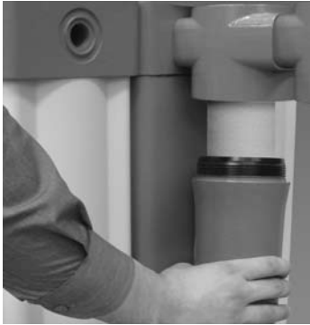
1. Unscrew and remove filter bowl from head.
