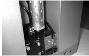
6. Locate diaphragm assembly to be changed.
