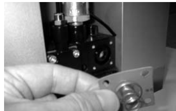
7. Remove diaphragm assembly.
