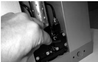
3. Remove bonnets by means of four fixing screws.
