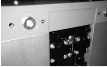
1. Remove the front panel and locate purge plug in upper valve block.
