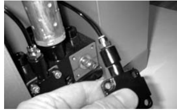
5. Disconnect tubing from fitting on bonnet.
