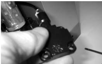
4. Separate bonnet from valve block.
