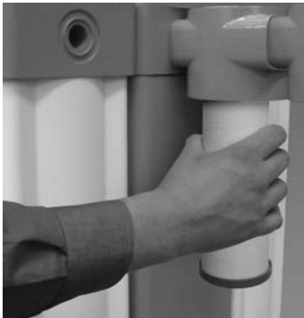
2. Remove filter element from head.
