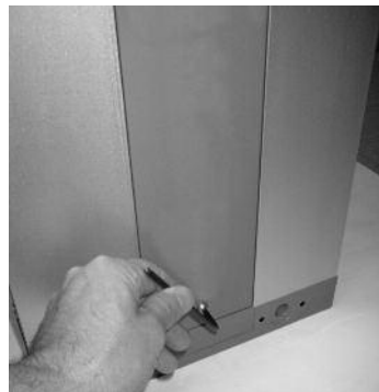
6. Replace single retaining screw.
