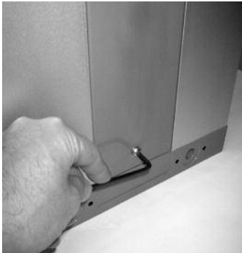
2. Remove single retaining screw.
