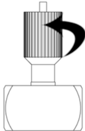
Turn knob clockwise (to the right) to close
